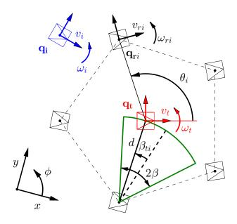
Fig. 1. Parameters involved in the problem formulation. Our contribution is the definition of the reference trajectories  $\mathbf{q}_{ri}$  for the robots  $\mathbf{q}_i$  to maintain a circular formation enclosing the target  $\mathbf{q}_t$  and maintaining FOV constraints. Each robot  $\mathbf{q}_i$  (only one is shown) will track its reference trajectory  $\mathbf{q}_{ri}$ . The FOV of the onboard fixed camera of one robot is also shown.
