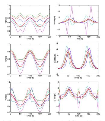
Fig. 3. Robot velocities of the first simulation in Fig. 2 enclosing and tracking a target with ellipsoidal motion. Three cases are shown from first to third row: Constant *d* not satisfying FOV constraint; constant *d* guaranteeing FOV; and maximizing *d*. Left column: Linear velocities  $v_{ri}$  and  $v_t$  (thicker). Right column: angular velocities  $\omega_{ri}$  and  $\omega_t$  (thicker) of all the robots.
