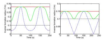
Fig. 4. Evolution of the inverse radius  $\kappa = 1/d$  for first (left) and second (right) example in Fig. 2. Strategy of constant d = 10 m ( $\kappa = 0.1$ ) not satisfying FOV constraint corresponds with the horizontal dashed line. Strategy of constant d guaranteeing FOV corresponds with the horizontal solid line. Strategy maximizing d corresponds with the Gaussian-like solid line. The curve in dashed line corresponds to constraint (14).
